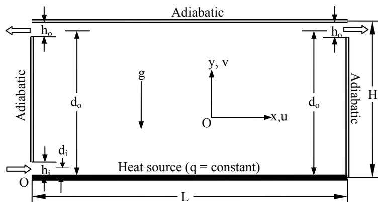
**Figure-1.** The geometry of the flow configuration under consideration, along with the coordinate system.
