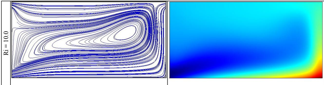
**Figure-4.** Streamline plots and contour map of temperature for different Richardson numbers at  $Re = 200$ .
