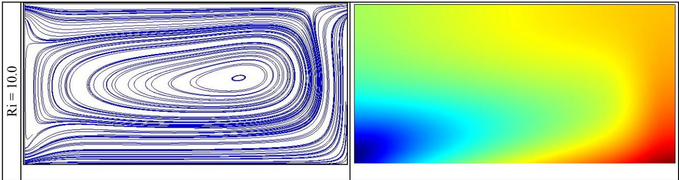
Figure-2. Streamline plots and contour map of temperature for different Richardson numbers at  $Re = 50$ .
