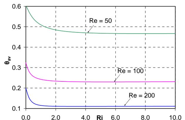
**Figure-5.** Variation of average dimensionless bulk fluid temperature with Richardson numbers.
