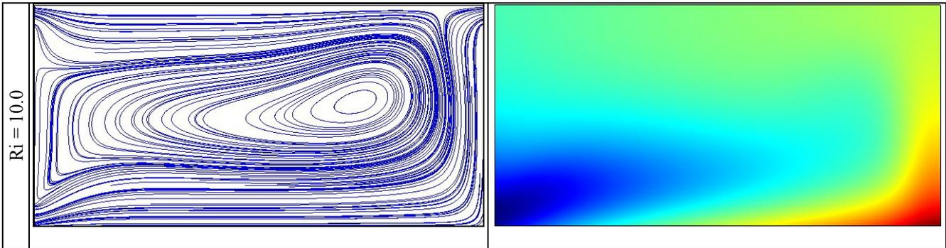
Figure-3. Streamline plots and contour map of temperature for different Richardson numbers at Re = 100.
