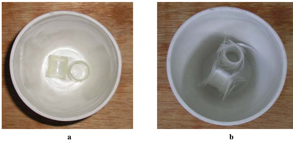
Figure-3. Specimen for volume fraction test (a) before burning (b) after burning.
