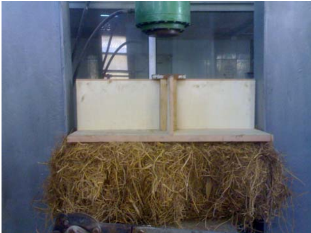
Figure-7. Hydraulic piston for compressing the bales and a wooden support for uniform load distribution on bales.
