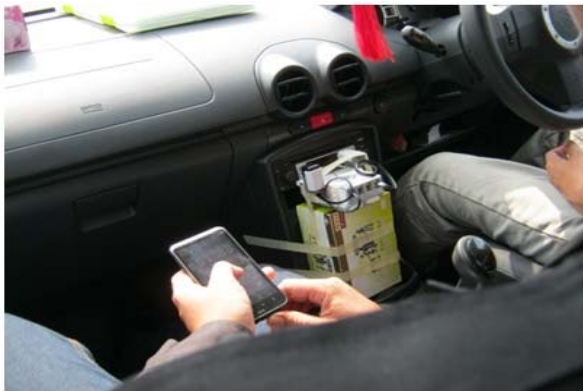
Figure-5. Location of DAQ in the vehicle.
